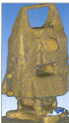
Figure 292. Ombrage plat du MNT © 3D Reshaper
